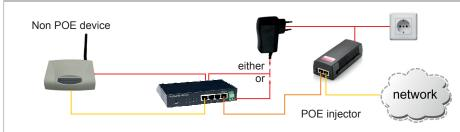
PingBrother \* has two or four 3-pol terminal blocks of Change-over relays. Using these, we can control the power of a non-PoE device or any other on/off controlled circuit. It is also possible to gain power from the POE input of the plug-in terminal block power connector of any equipment (PoE power separator function). For the EPIW104P an optional moisture sensor is available wich can switch or send an email in case of water leakage or condensation.
