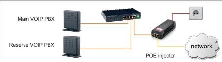
PingBrother \* can work as a fail-over backup controller. This means that it can switch to a reserve equipment in case of a device error. If you have a very important service running on your device, and you set up a reserve with the same services, even on the same IP address, PingBrother can turn the faulty one off and the reserve one on in case of a failure. The controlled equipment can be PoE or non-PoE device as well.
