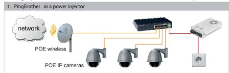
PingBrother \*receives power from a plug-in terminal block connector, and powers all the connected devices (max. 4) over an ethernet cable. Power supply output must be calculated according to the total current load of the connected PoE devices. In case of a failure, PingBrother automatically reboots the dysfunctional equipment. It writes a log entry about its action and if set, sends an e-mail.
