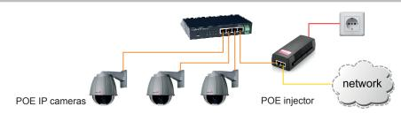
PingBrother \* receives power through its own first ethernet port and powers all the connected devices (max. 3) over an ethernet wire. Power injector output must be calculated according to the total current load of the connected POE devices. In case of failure automaticly reboots the dysfunctional equipment. It writes a log entry about its action and if necessary sends an email. Manual remote management is also possible (on, off, reset) via network or Internet.
