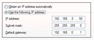
Click **Apply** and close windows. Ping the power switch to confirm the connection. Point your browser at 192,168,0,100 and log in. Find detailed instructions at digital-loggers.com/ip\_setup.html
