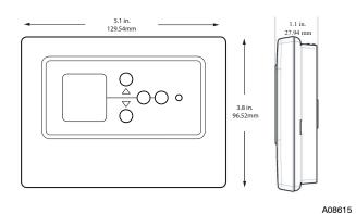
Fig. 6 - Legacy Line Series Standard Screen Non-programmable
