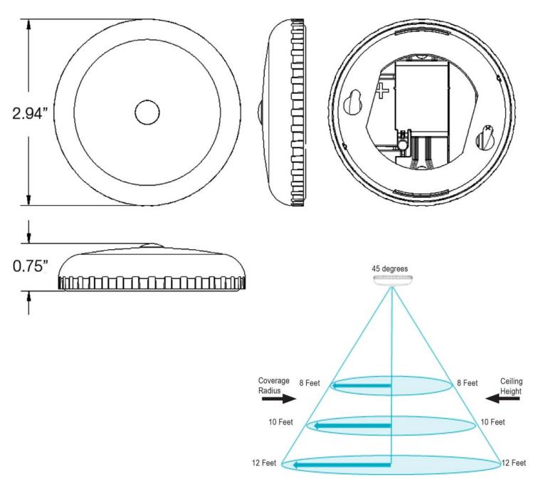
Note: Position the ceiling motion sensor for best use of its detection zones. All measurements are approximate and will vary with installation.
