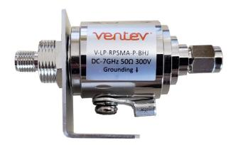
Ventev's Lightning Arrestor is a bi-directional gas discharge tube suppressor that features wide-band operation up to 7 GHz and is rated at IP67. Simply attach the lightning protector to an access point to help protect an entire network, outdoor antennas, and other wireless equipment from the build-up of static electricity. It is recommended to use 11 American Wire Gauge (AWG) ground wire.
