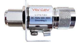
Ventev's Lightning Arrestor is a bi-directional gas discharge tube suppressor that features wide-band operation up to 7 GHz and is rated at IP67. Simply attach the lightning protector to an access point to help protect an entire network, outdoor antennas, and other wireless equipment from the build-up of static electricity. It is recommended to use 18 American Wire Gauge (AWG) ground wire.
