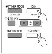
Press the DAY (DAY OFF) button and TIMER SET button simultaneously for 2 seconds or more to activate the part lock function and lock all of the buttons on the remote controller except the START/STOP button, "& SET TEMP. ♥" "I SET TEMP. A" buttons, "(⊗\*0 MODE" button, and "% FAN" button. Press the buttons again for 2 seconds or more to deactivate the part lock function.
