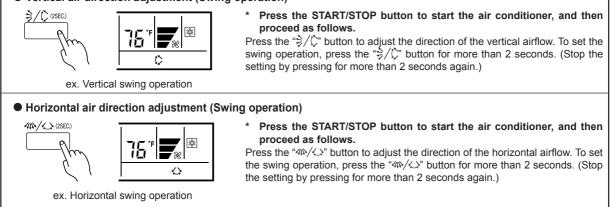
• Each time the button is pressed, the airflow direction setting changes as shown in MANUAL OPERATION which is included in IN-DOOR UNIT.
