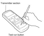
To end test operation, press the remote controller START/ STOP button.
