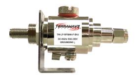
Ventev's TerraWave lightning arrestor is a bi-directional gas discharge tube suppressor that features wide-band operation up to 6 GHz and is rated at IP67. Simply attach the lightning protector to an access point to help protect an entire network, outdoor antennas and other wireless equipment from the build-up of static electricity. It is recommended to use 18 American Wire Gauge (AWG) ground wire.
