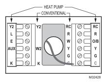
Connect the common side of the transformer to "C" terminal. This connection is mandatory.
