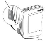
The thermostat is shipped from the factory with the coin cell installed. To keep the battery from discharging during shipment and storage, the thermostat is shipped with a plastic tab inserted in the battery holder. This tab must be removed during installation. Simply pull the plastic tab out of the battery tray. Make sure that the battery tray is fully inserted into the thermostat.
