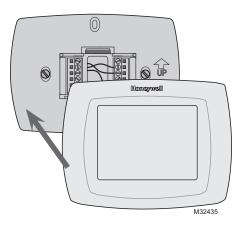
Align pins on back of thermostat with slots in wallplate, then push gently until thermostat snaps into place.
