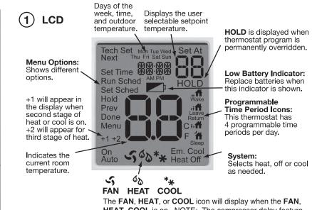
The **FAN**, **HEAT**, or **COOL** icon will display when the **FAN**, **HEAT**, **COOL** is on. NOTE: The compressor delay feature is active if these icons are flashing. The compressor will not turn on until the 5 minute delay has elapsed. These may also flash for staging delay or floor sensor override.
