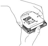
To remove the thermostat backplate: Gently separate the display from the base by pulling first from one side, then the other until the two pieces unsnap. A small screwdriver may be used, very carefully, to start seperating the two pieces.
