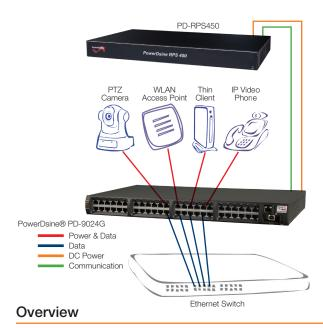
The PowerDsine(R) Redundant Power Supply (RPS) increases reliability for data, voice and video networks by ensuring reliable safe power for all PoE applications including VoIP, wireless LAN, IP security cameras, thin clients and other end terminals.
