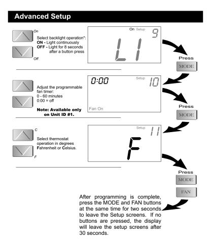
\*For increased battery life the backlight should be set to OFF unless the P474-0800 RF power supply adaptor is used to power the thermostat.
