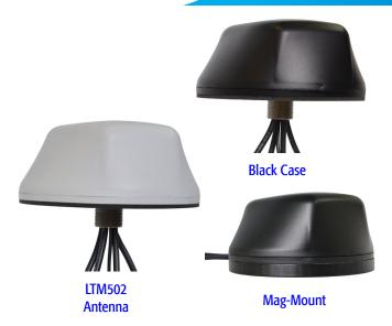
Mobile Mark's LTM502 Series antenna contains five separate antennas, all in one compact antenna housing: two broadband LTE/Cellular antennas, two dual-band WiFi antennas, and one GPS antenna. The LTM502 differs from the LTM501 in that the broadband LET/Cellular element covers all LTE frequencies worldwide, from 694-3700 MHz.
