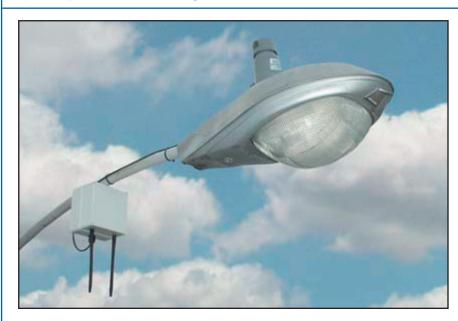
The PoE OWL provides power through a user specified cable and user specified connector for ancillary devices. The input power comes from a standard NEMA Street Light receptacle. Any line voltage up to 480 VAC is converted to user specified DC voltage.
