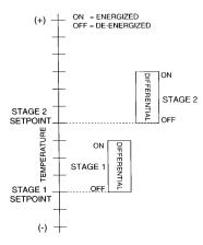
Figure 2: Two Stage Cooling Example
