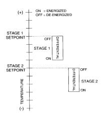
Figure 1: Two Stage Heating Example
