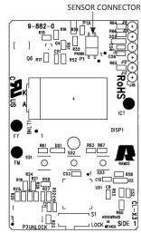
Figure 9: Sensor replacement on Display (Upper) Circuit Board.
