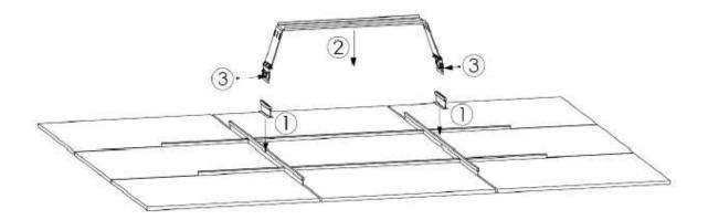
Sample installation: 1. Assemble insulating labels on ceiling rails. 2. Snap lock holder to ceiling rails. 3. Secure installation with 2pcs Nylon screws
