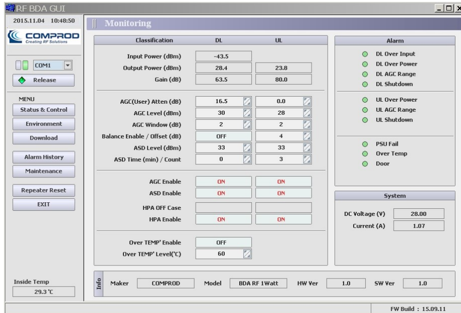
Visual Alarms and Remote Failure Monitoring with Graphical User Interface
