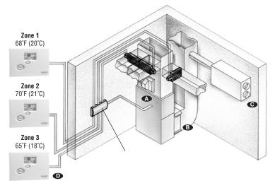
The above illustration shows a typical three zone Aprilaire Zoned Comfort Control system with the following Research Products Corporation components added for the ultimate in indoor air quality and comfort:
