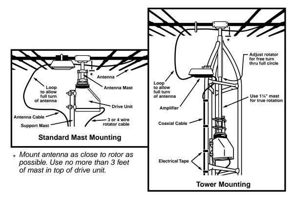
*Do not mount citizens band base station antennas on top of a standard mast mount drive unit. Mast support may become overloaded in high winds.*
