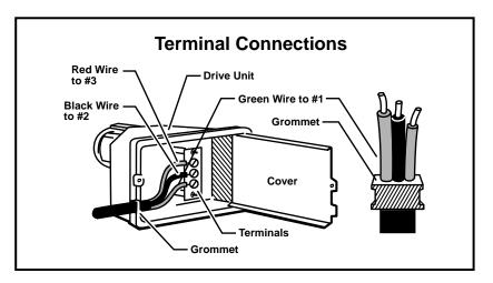
Caution – Make sure bare connectors do not touch. It is suggested that the screws and bare conductors be painted with nail polish after cable is connected. To avoid moisture collecting in the cable be sure jacket of cable passes thru the grommet.
