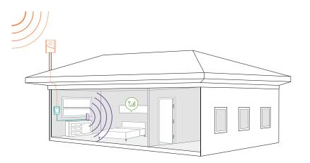
**Receives signal:** The powerful antenna reaches out to access voice and data signals, and delivers it to the booster.
